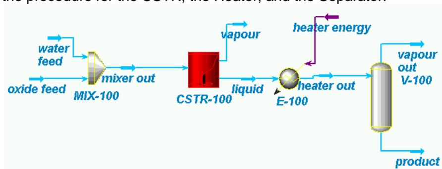
We need to specify the parameters of the two feed streams, their temperatures, pressures, flow rates, and compositions.
