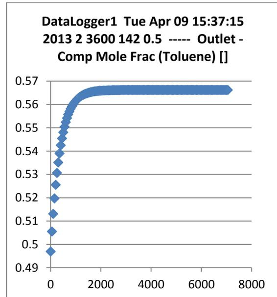
Note that the Time column begins at 0.5s. This is important. If you have a time offset in your excel data you will need to recalibrate this by subtracting the ~initial time from all the values in the Time column.
