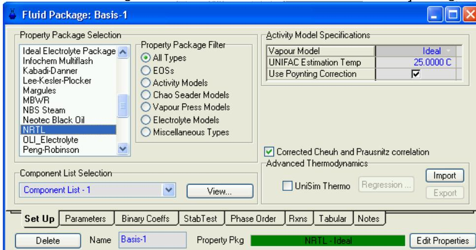
Check on the Binary Coefficients tab that the two interaction parameters have been successfully calculated (they should be in red type).
