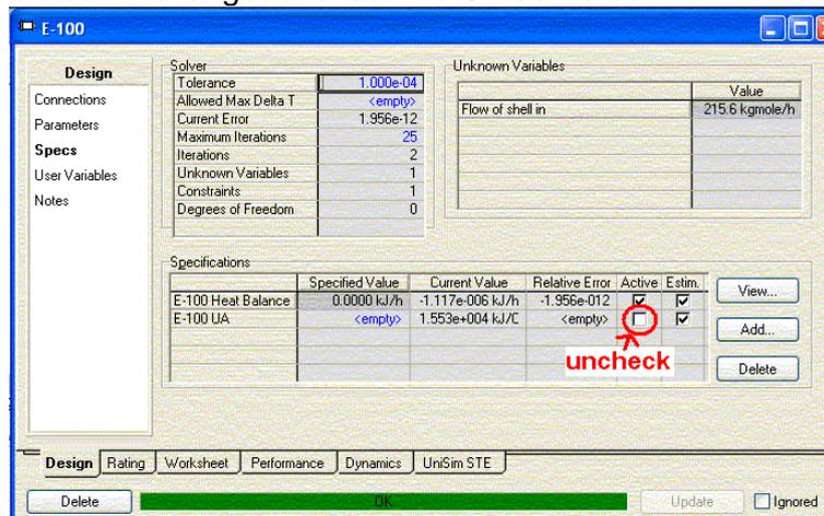
We have now specified seven of the nine parameters a heat exchanger needs, and this is enough to solve it uniquely. It's smart enough to figure out the composition of the outlet streams, and to calculate the flow rate through the shell and the UA value for the heat exchanger.
