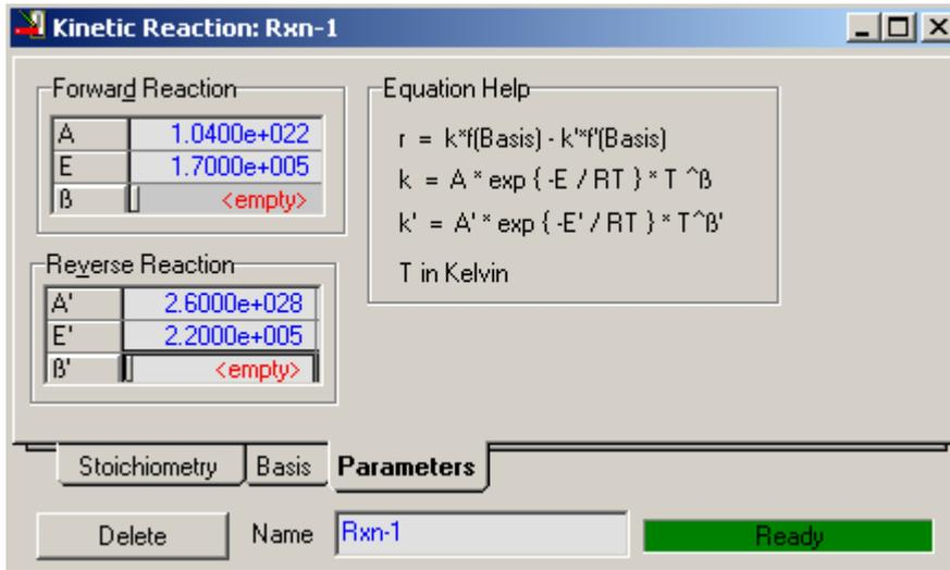
Once this is done you can close the Kinetic Reactions window. Then you must press *Add to FP* on the *Reactions tab* of the *Simulation Basis Manager* (this is shown in an image above).
