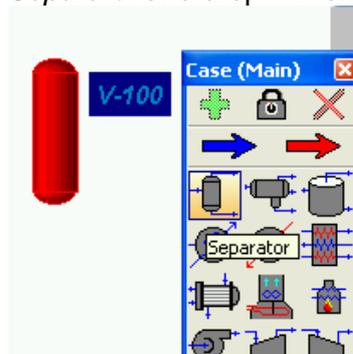
Double click on the new separator vessel, V-100, to enter its dialog box
