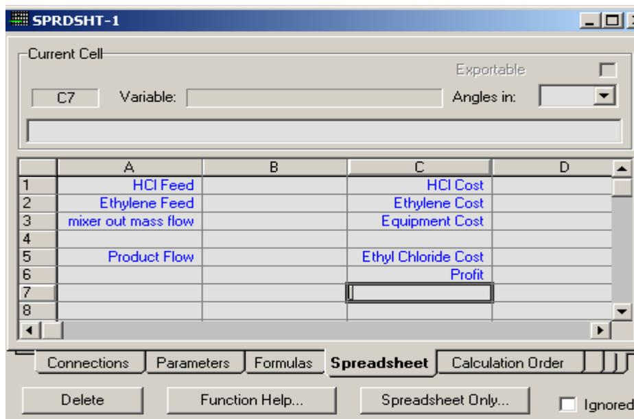
Right click in cell b1, chose Import Variables, FEED, Comp Mass Flow, HCl. Do the same for cells b2, b3, and b5 with the appropriate choice of variable. It should give you a spreadsheet as follows:
