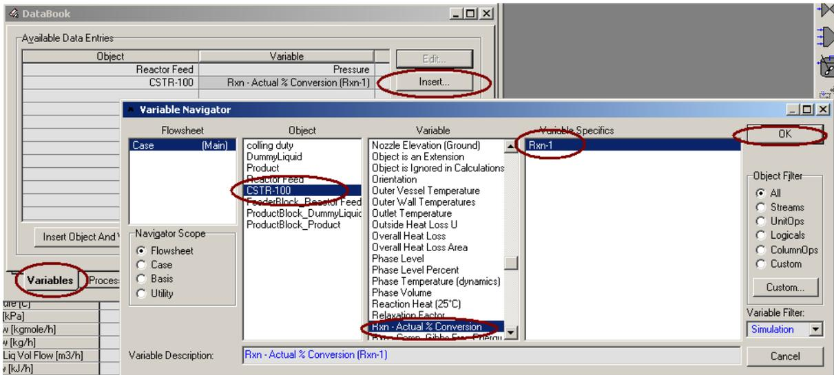
On the Case Studies tab Add a new case study and choose the Reactor Feed Pressure as the independent variable and the CSTR Rxn – Actual % Cnv as the dependent variables as shown below
