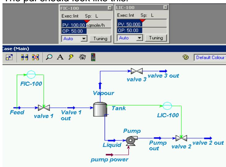
Your next job is to add a third controller to control the tank pressure level (called here *Vessel Pressure (dynamic specification)*). A range of 300-700kPa seems OK, and a  $K_c = 2$  would work. We'll leave it a proportional only controller so leave  $T_i$  and  $T_d$  empty. But you'll need to find the correct PV, select the appropriate OP, and decide if it's direct or reverse acting.
