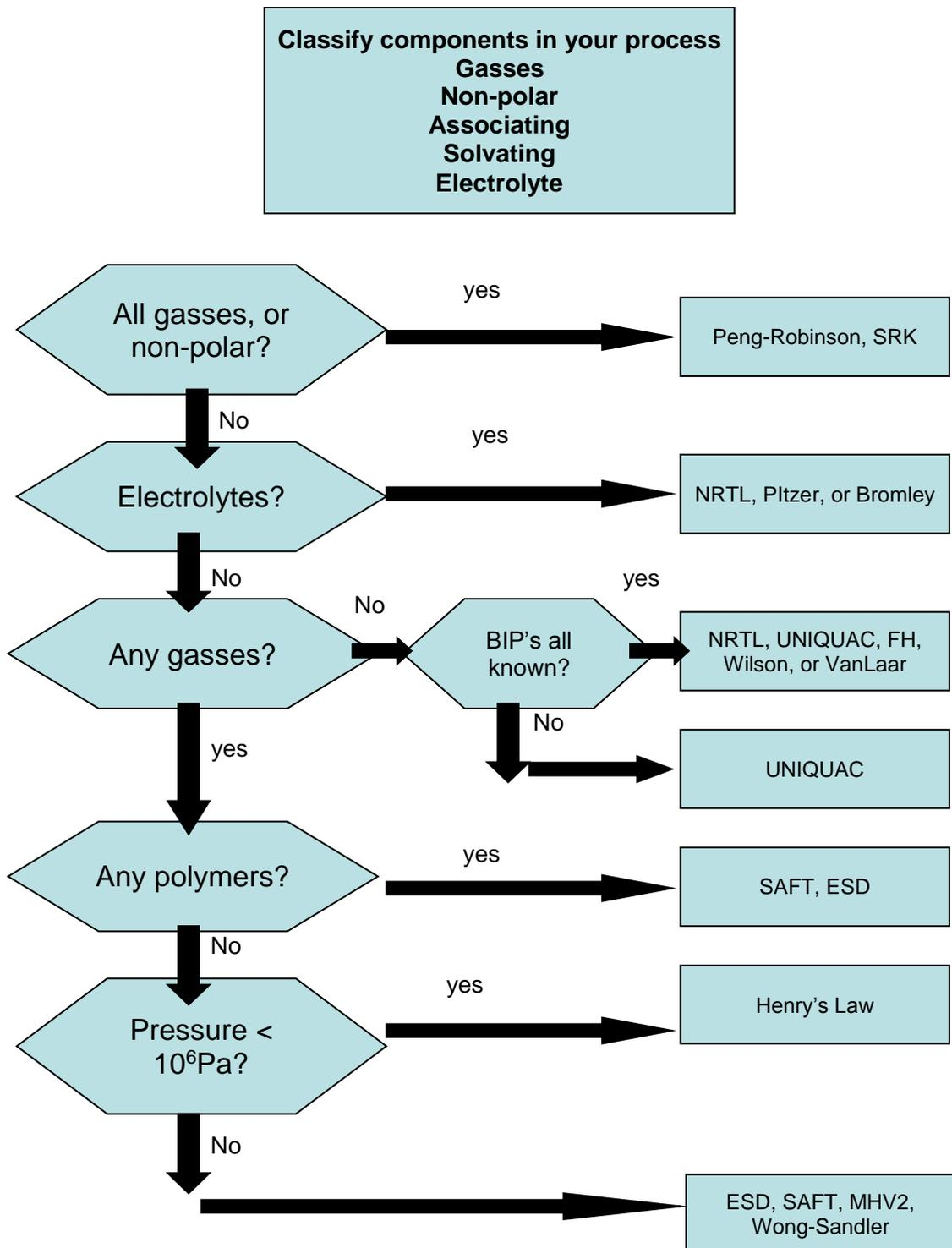
The connection between temperature and pressure will depend not only on what chemicals are present but also on how they mix together. For this we need the binary reaction coefficients.
