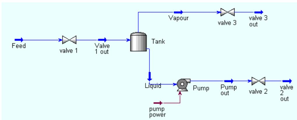
Now we need to prepare our simulation for the switch into dynamics mode. This is important because some factors, like for instance the tank size, have no impact on the steady state conditions but are critical to know when it comes to the time response of the system, its dynamics.
