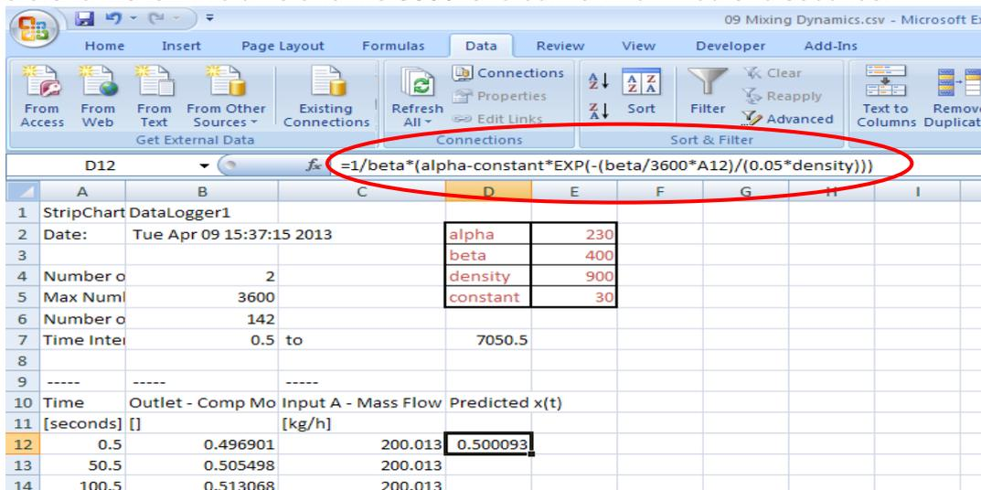
Having done this for one cell, you can copy this formula for every subsequent cell (i.e. *Fill, Down*). The fastest way to do this is to left click the bottom right corner of the first cell, drag down over the column, and then chose copy cell. See the diagrams below for before and after.
