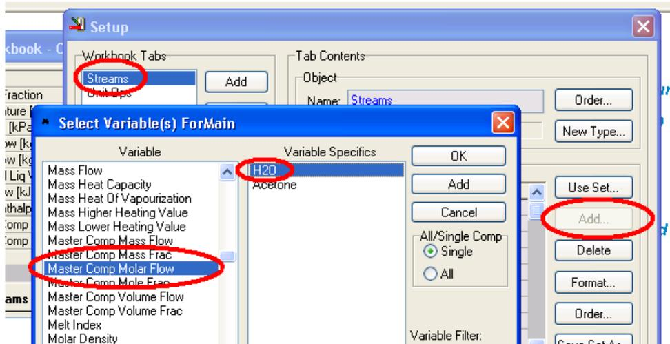
Examine the output from the workbook and verify that material balance is good for total molar flow, and for each component molar flow fraction.
