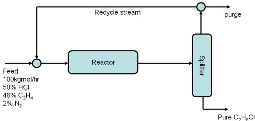
Since the reaction only achieves 90% conversion the unreacted components are separated from the ethyl chloride and recycled.
