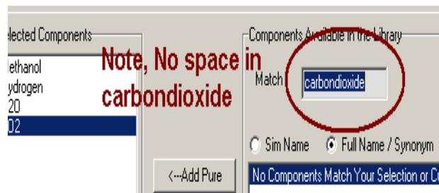
Click *Add* and then add methanol, water, hydrogen, and carbon dioxide to the components list. Using the *Match* search box helps a lot here.
