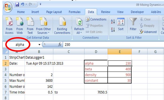
We are now going to create a new column in our excel sheet for the predicted value of x(t) and fill it out with values based on our equation. Do this as shown below. Note, the 0.05 refers to the tank volume and the 3600 is to convert from hours to seconds.
