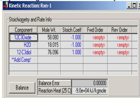
Next, select the Basis tab of the Kinetic Reactions pop-up and change the Base Component from H<sub>2</sub>O to PropOxide and also change the Rxn Phase to Combined Liquid. Change the Basis Units to lbmol/ft<sup>3</sup> and the rate units to lbmol/ft<sup>3</sup>-hr. Then click on the Parameters tab to input the Arrhenius parameters for the reaction. Type in 1.7e13 for the forward A parameter and 75362 for forward parameter E. There is no reverse reaction
